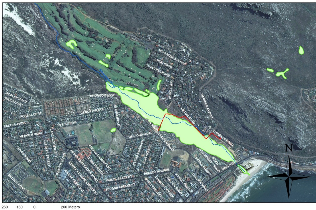
Figure 2 2010 aerial photograph showing the proposed alignment of the electrical cable, in its extent through the Silvermine River and its associated wetlands only. Wetland extent shown as green polygons, as mapped by the City of Cape Town' (2009) GIS layer. Low flow channel of the Silvermine River shown as blue line.
