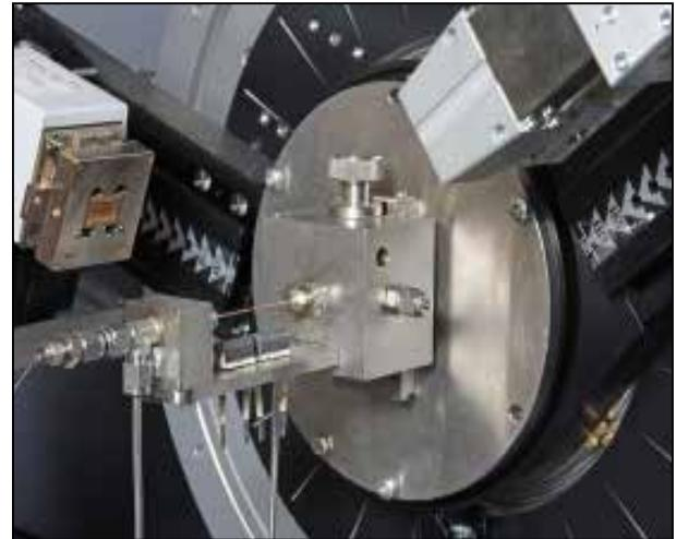
This uniquely designed *in situ* reaction cell can be mounted on any commercial XRD and it can be used both with conventional diffractometers and in conjunction with synchrotron facilities.
